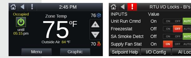
Setpoint Help ₲ ◀ Supply Air Temp Setpt Default Value: 00 °F When a building's supply fan(s) system Δ is operational, the discharge-air temperature setpoint value should be automatically adjusting to internal/external conditions that will allow the supply fan to operate more efficiently. When the set point values are
